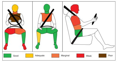
Figure 21: Dummy Injury Diagrams of Driver and Passenger in Frontal Test and Driver in Side Test
