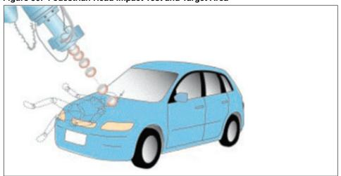
Figure 50: Pedestrian Head Impact Test and Target Area
