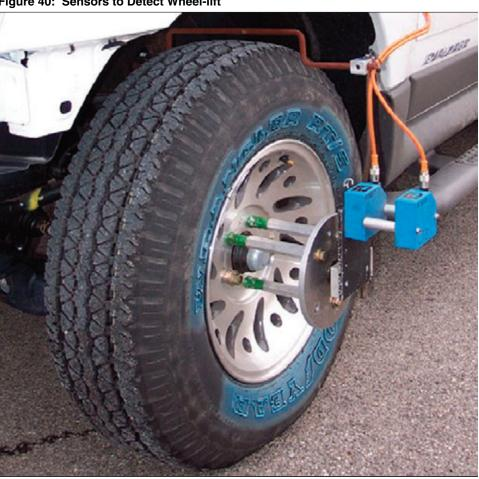
Figure 40: Sensors to Detect Wheel-lift
