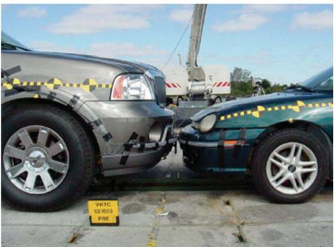
Figure 27: Example of Improved Matching of Frontal Vehicle Structures
