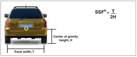
Figure 9: Calculation of a Vehicle's Top-Heaviness
