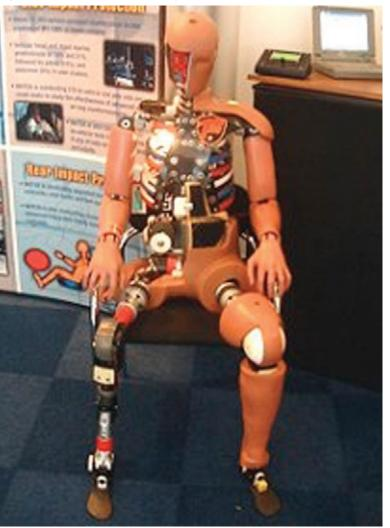
Figure 32: A Crash Test Dummy Fitted with Load Sensors and Accelerometers
