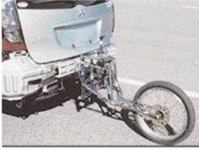
Test vehicle is equipped with a device for measuring stopping distance and vehicle speed.
