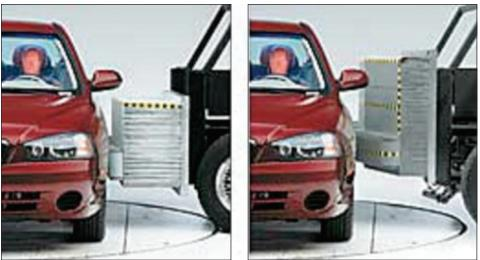
Figure 16: Comparison of Barriers Used in the NCAPs' Side Test (left) and the Insurance Institute Side Test (right)
