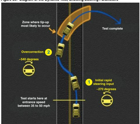
Figure 39: Diagram of the Dynamic Test, Showing Steering Parameters
